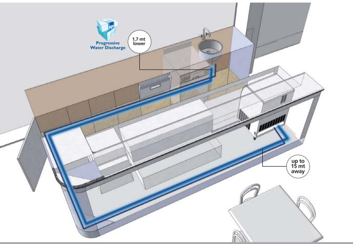
PWD - (Progressive Water Discharge) is the smart, pressurized discharge system that will allow you to reach remote water drains to dispose of the left over water at the end of each production cycle, as well as the water resulting from the ice melting over time in the storage bin. A non-return valve prevents any potential drain water back-flush into the system, greatly improving the overall hygiene of the ice machine.
